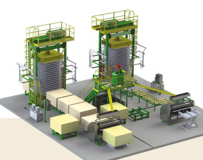
Full set of equipment for laminating the plywood from peeled veneer.
